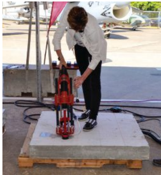
Managing Editor Elizabeth Manning recently attended Hilti's Innovation Day, where she and other media representatives in attendance had the chance to test the usability of Hilti's new DD30-W diamond core drilling system (pictured here). The drill increases accuracy and is exceptionally quiet, making it a great solution for jobs where loud hammer drilling is prohibited.
